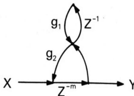
Figure 4.9: Comb filter with a one-pole filter in the loop. [Moorer, 1979]
