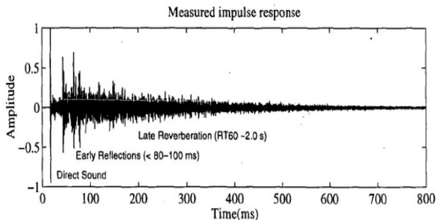
Figure 3.1: Typical RIR of a room [Savioja et al., 1999].
