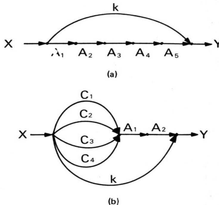
Figure 4.8: a) Series combination of All-pass filters  $A_i$ , b) Comb filters  $C_i$  in parallel and two All-pass filters in series. Here  $k$  denotes the gain factor for direct sound [Moorer, 1979]
