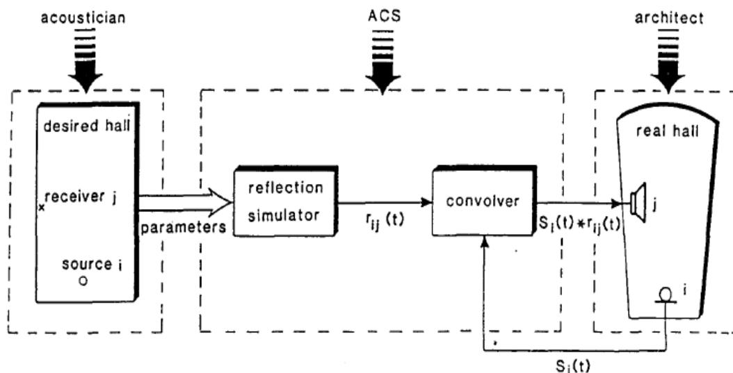
Figure 5.8: Principle of ACS for one loudspeaker pair [Berkhout, 1988].
