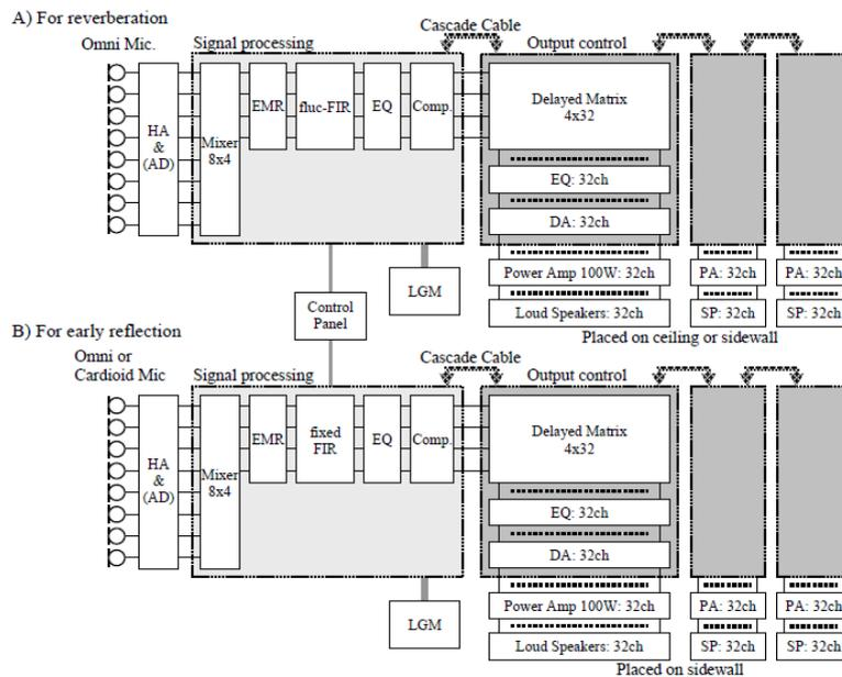
Figure 5.7: *Block diagram of AFC* [Miyazaki, 2003].
