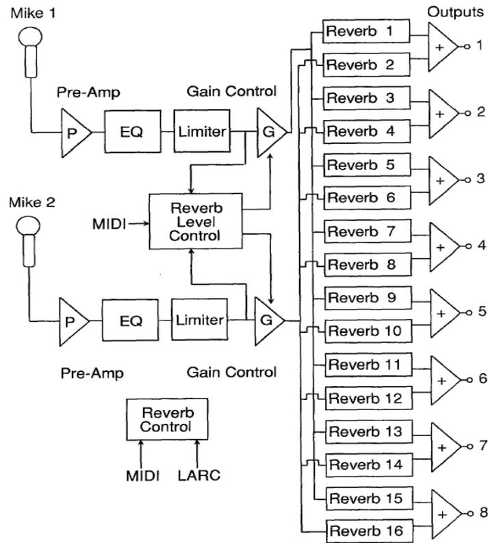
Figure 5.10: *LARES Block Diagram of the Elgin System [Griesinger, 1991].*
