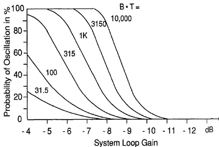
Figure 4.3: Probability of Oscillation with a distinct loop gain and bandwidth [Schroeder, 1954].
