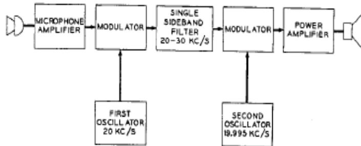
Figure 4.4: Block diagram of a frequency shifter. [Schroeder, 1959]
