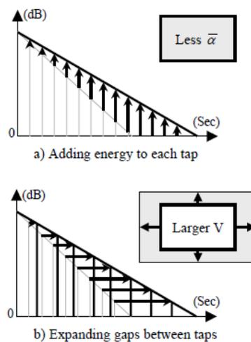
Figure 5.6: *FIR filter control possibilities* [Miyazaki, 2003].
