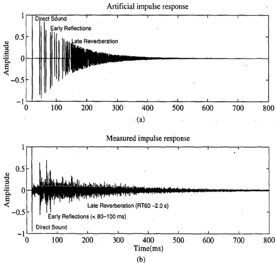
Figure 4.15: a) *Simulated Impulse response of a room* b) *measured IR.*
