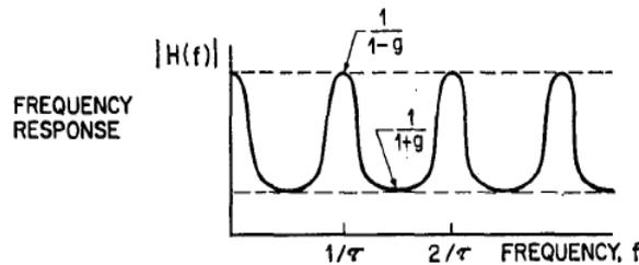
Figure 4.7: Frequency response of a comb filter. [Schroeder, 1962]
