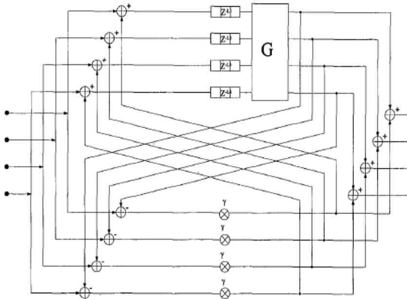
Figure 5.13: *Block diagram of unit reverberator [Poletti, 1996].*
