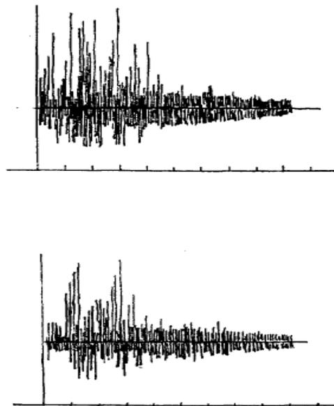
Figure 5.11: *Impulse response of one reverberator. One minute apart [Griesinger, 1991].*
