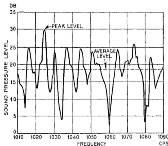
*Figure 4.2: Section of a frequency response of a room. CPS means cycles per second. [Schroeder, 1959]*
