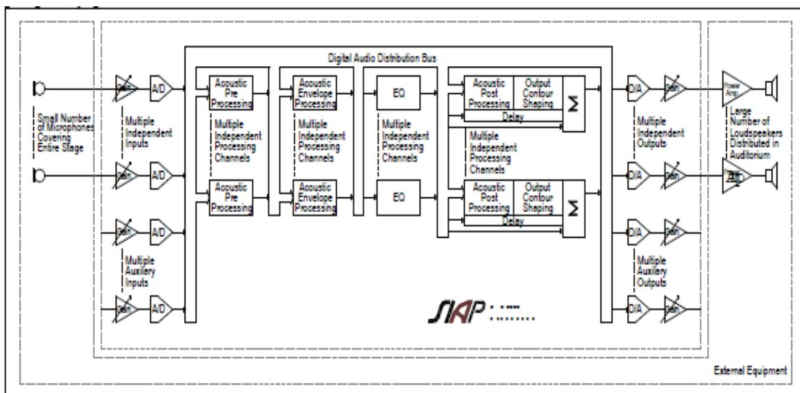
Figure 5.14: Concept of SIAP system [Kok and Prinssen, 2009].
