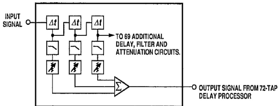
Figure 5.4: *Simplified 72-Tap Delay Processor Schematic* [Jaffe, 1992].
