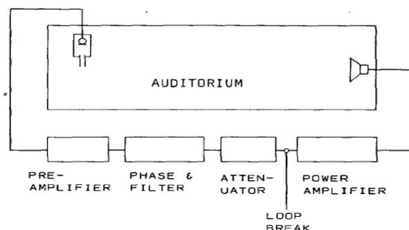
Figure 5.1: *Components of a Assisted Resonance channel [Parkin, 1970].*
