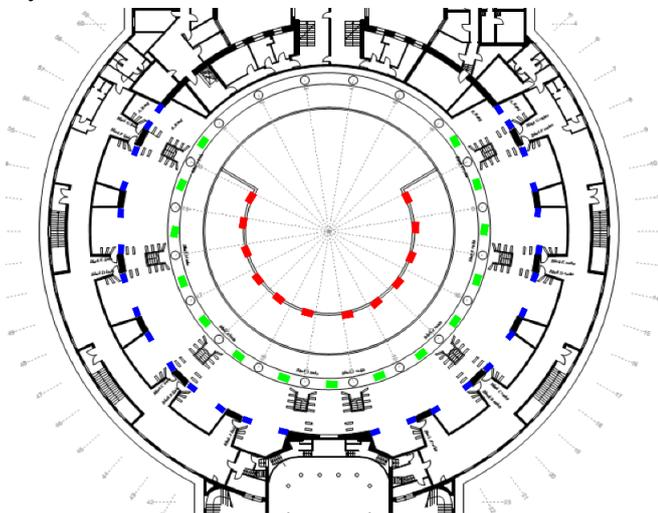
**Fig. 9:** Layout of loudspeakers in the Kuppelsaal Hannover.
