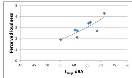
**Figure 7:** Regression model of the measured equivalent continuous sound pressure level and the perceived loudness.
