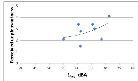
**Figure 8:** Regression model of the measured equivalent continuous sound pressure level and the perceived unpleasantness.
